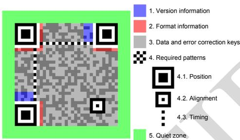
Fig. 2. Different structural parts of a QR code.
